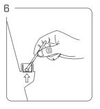
Use loading tool or a Puffco Dual Tool to place contents on the bottom surface of the bowl (not the sides).
