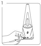
Fully charge the device before first use. The lights will pulse white while charging. The Peak Pro Power Dock can wirelessly charge your device. (sold separately)
