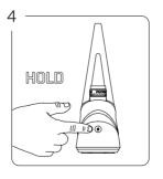
To unlock / lock the device, hold down the button for 3 seconds. (Preserves battery between uses)
